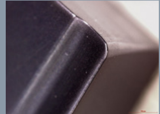
Edge of cutting tool taken with 3D-microscope
